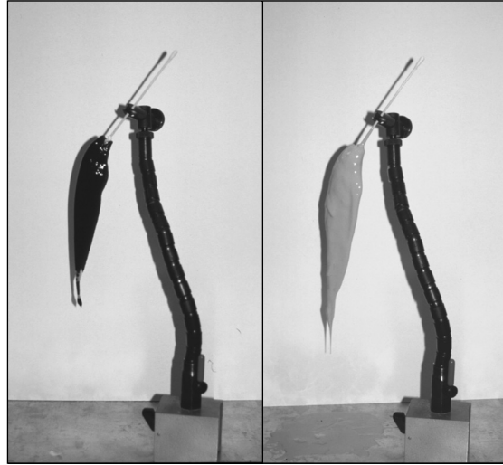
Figure 3.1 Making an RTV silicone mold of a weakly electric fish. (A) The support rod is positioned so that the dorsal curvature of the fish approximates the natural posture in water. (B) During casting silicone is slowly poured on the fish until it covers the entire surface. Several layers of casting compound are added, with enough time between layers for the silicone to partially cure.
