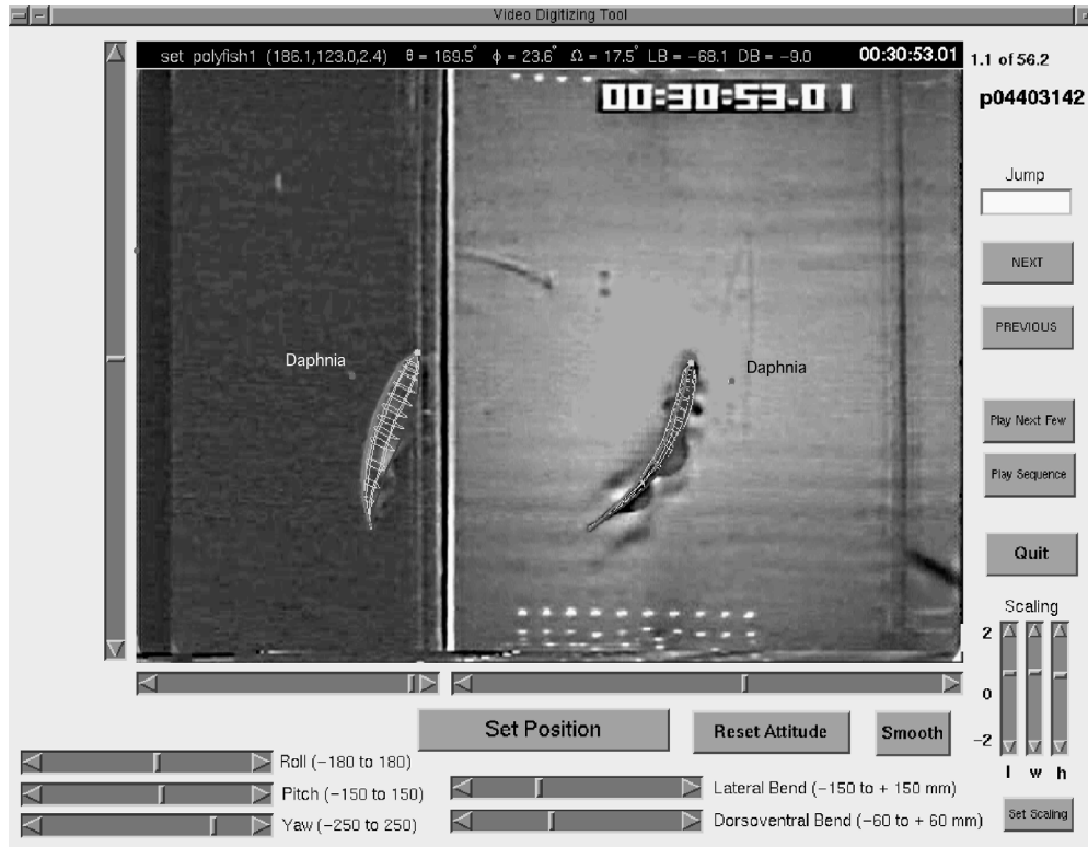
Figure 3.6 Snapshot of the animal tracking interface. The sliders adjacent to the image control the (x, y, z) position of the snout; the sliders below control yaw, pitch, roll, lateral bend, and dorsal-ventral bend. The scaling sliders control the subject-specific scaling of the polygonal model. The user navigates through the fields of the behavioral sequence and manipulates the polygonal model so that its top and side viewport projections are congruent with those of the real fish.
