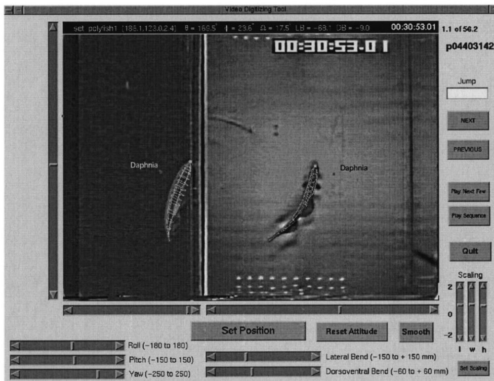
Fig. 6. Snapshot of the animal-tracking interface. The sliders adjacent to the image control the (x, y, z) position of the snout; the sliders below control yaw, pitch, roll, lateral bend, and dorsal-ventral bend. The scaling sliders control the subject-specific scaling of the polygonal model. The user navigates through the fields of the behavioral sequence and manipulates the polygonal model so that its top and side viewport projections are congruent with those of the real fish.
